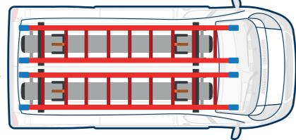
The G2000 Harrier's ladders holding system can be upgraded for holding 2 x extension ladders on each equipment by stacking them.
