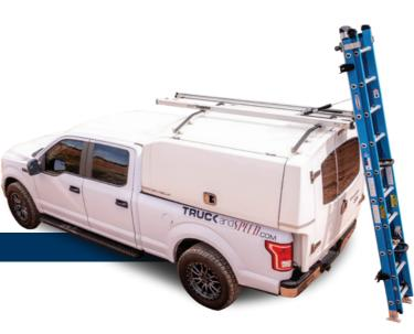
With the G2000 series, health risks to the back and shoulders are dramatically reduced when loading / unloading long and heavy ladders because the operations are assisted by a hydraulic assistance system reducing the effort required to a minimum.
